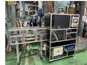
Newly introduced AI-based image inspection system
